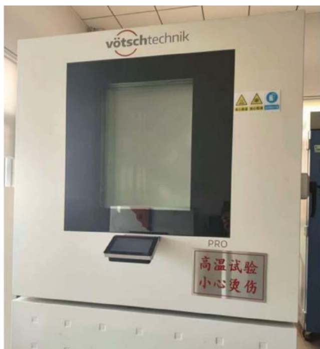
FIGURE 1 Environmental temperature test chamber.
