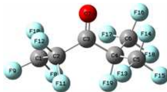
Fig. 3. Schematic diagram of C 6 F 12 O molecular structure.
