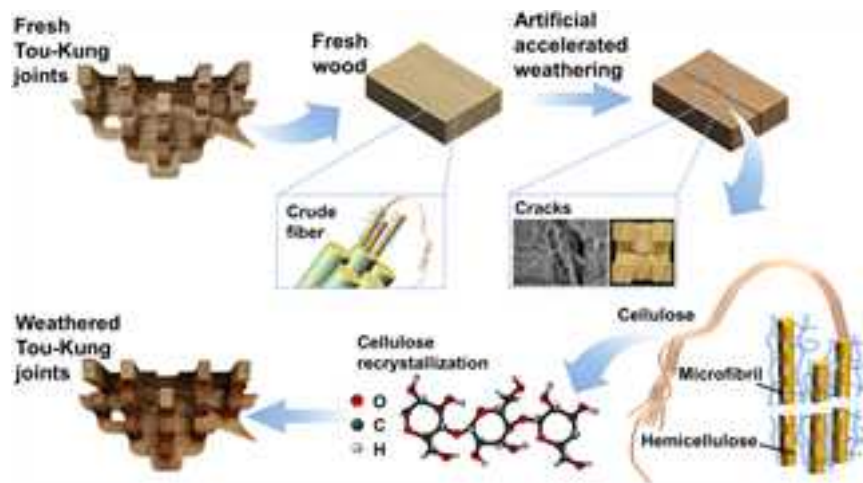
Fig. 15. Schematic diagram illustrating the degradation mechanism of Tou-Kung joints mechanical response at weathering conditions.
