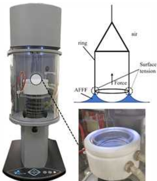
Fig. 4. The figure of surface tensiometer and testing principle.
