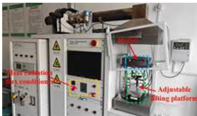
FIGURE 1 The cone calorimeter and testing platform.
