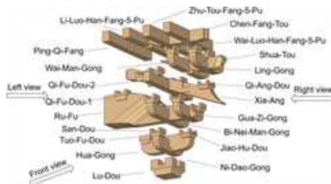
Fig. 2 | Configurations of Tou-Kung.
