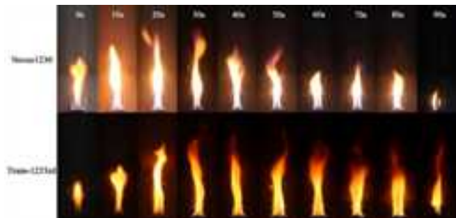
Fig. 2. Flame patterns of pure Novec1230 and tran-1233zd in action.
