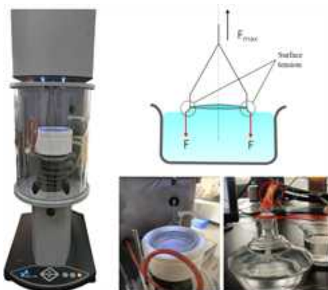
Fig. 4. Surface tensiometer and testing principle.
