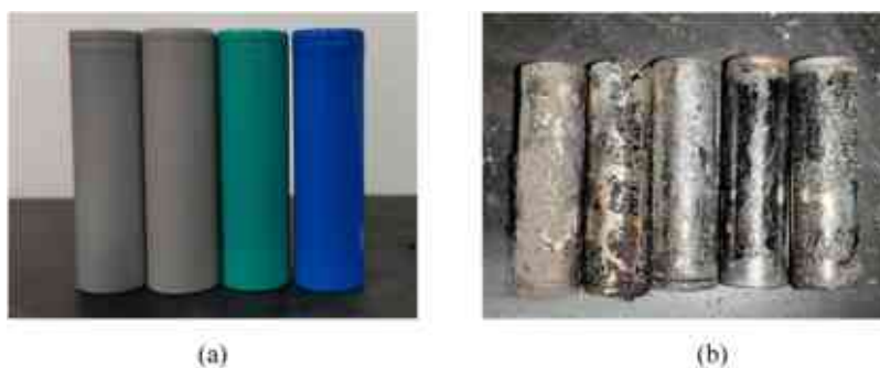
Figure 4. Description of LIB samples (a) prior to test (b) after test.
