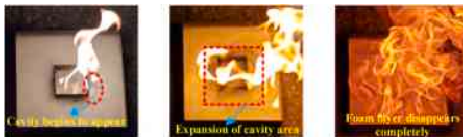
Fig. 20. The shape of the foam layer at different stages.
