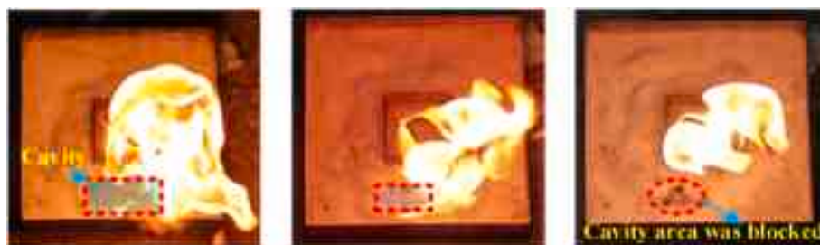
Fig. 22. Spreading process of the foam on oil surface.
